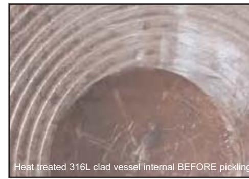
Heat treated 316L clad vessel internal BEFORE pickling
